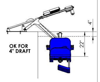
ADJUSTED ALL THE WAY UP USE FOR WATER DRAFT UP TO 4"
