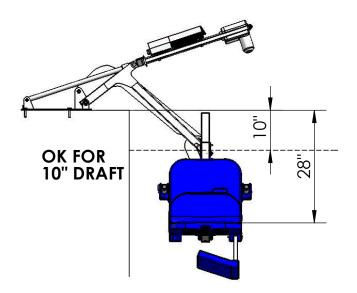
ADJUSTED ALL THE WAY DOWN USE FOR WATER DRAFT UP TO 10"
