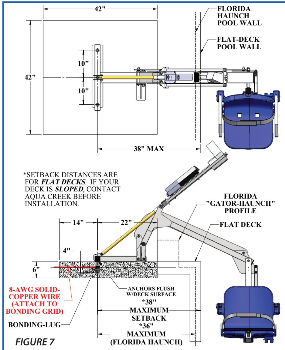
The footing for the lift should be tied into the rest of the pool deck on three sides with the rebar or reinforcing mesh. (Do not tie into the bond beam). The rest of the pool deck can be a typical 4" thick or thickened per local code requirements. Bond rebar or reinforcing mesh grid according to local requirements and also bond the anchor system to the rebar/mesh grid.
