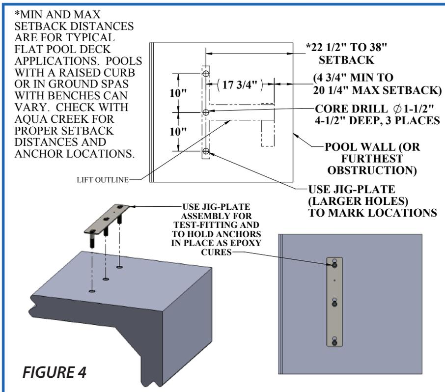
12. Allow the epoxy to set up according to the manufacturer's recommendations and remove the hardware and the anchor jig-plate. The lift can now safely mount to the anchors using the same hardware used to mount the anchor inserts to the underside of the anchor jig-plate. The anchor jig-plate can be recycled or used for installing a second set of anchors in another location.
